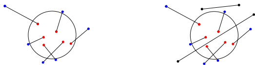
Figure 1: Left: Segment set with a stabbing circle. Right: Segment set with no stabbing circle.
