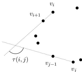
Figure 1: Turning angle.
